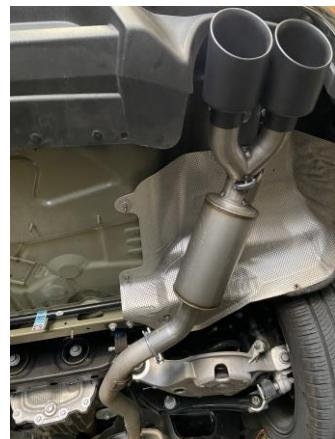
1. First you'll need to cut both tailpipes 1.5" from the beginning of each straight closest to the muffler, the cuts are marked in this photo. (**BE SURE YOU CUT CORRECTLY**). Once cut you may remove both muffler assembly's and clean the burr on both pipes that are still on the vehicle.
