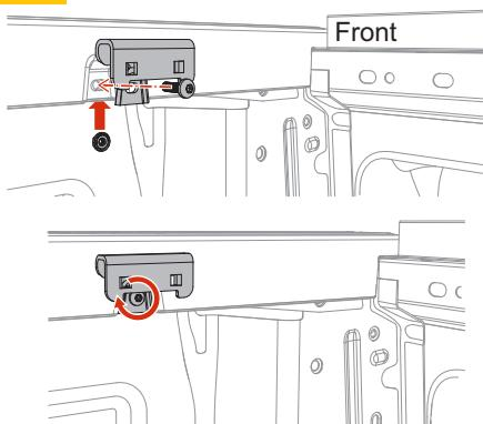
Place the front (cab) latch bracket into the front recess in the truck bed rail. Thread the screw through the bracket, through the bed rail and into the nut. With a wrench and Torx tool tighten the screw. Install on both sides.
