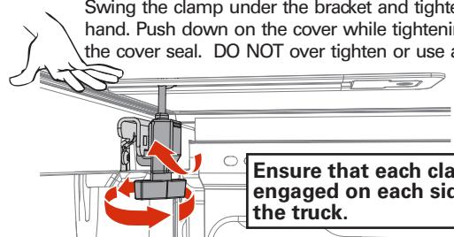
Ensure that each clamp is engaged on each side of the truck.
