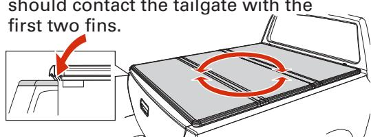
**7** Carefully refold the bed cover without shifting its position on the truck bed.
