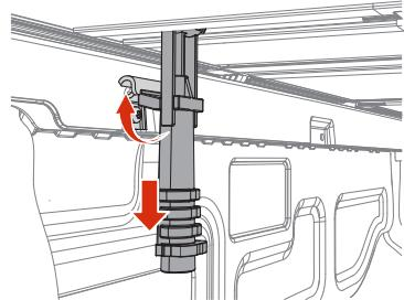
Ensure that each clamp is engaged on each side of the truck.
