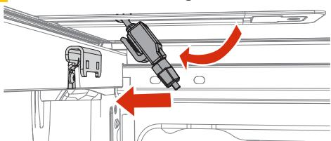
Rotate the body of the clamp up or down to match its position with the bracket.
