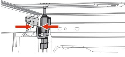
Swing the clamp under the bracket and tighten by hand. Push down on the cover while tightening to help the cover seal. DO NOT over tighten or use a wrench.
