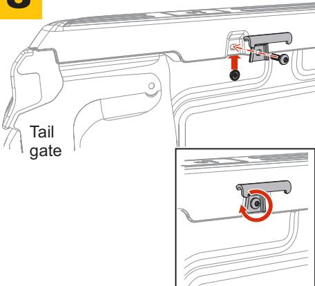
Place the rear (tailgate) latch bracket into the rear-most recess in the truck bed rail. Thread the screw through the bracket, through the bed rail and into the nut. With a wrench and Torx tool tighten the screw. Install on both sides.
