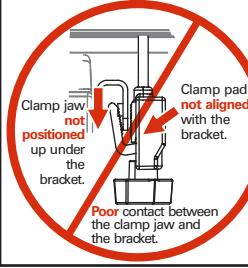
The optimal position of the clamp body is to match the bottom of the ridges to the bottom of the bracket.
