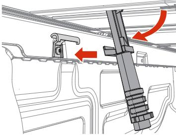
Pull the clamp down and hook it under the bottom edge of the rear bracket.
