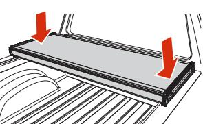
**6** Unfold the bed cover fully and adjust the position over the truck bed for proper front (cab) and rear (tailgate) alignment. When positioned front and back, the tailgate seal should contact the tailgate with the first two fins.
