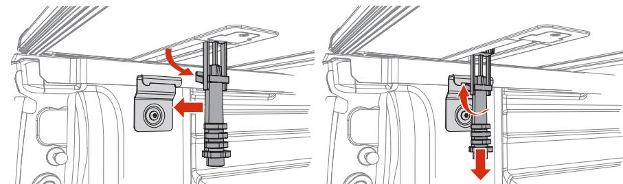
Pull the clamp down and hook it under the bottom edge of the rear bracket.
