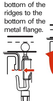
Swing the clamp under the bracket and tighten by hand. Push down on the cover while tightening to help the cover seal. DO NOT over tighten or use a wrench.
