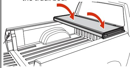
**4** Slide the front (cab) clamp at an angle toward the bed rail and swing it down.
