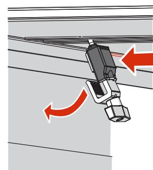
Rotate the body of the clamp up or down to match its position with the bed rail flange.
