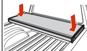
**2** Unfold the bed cover fully and adjust the position over the truck bed for proper front (cab) and rear (tailgate) alignment. When positioned front and back, the tailgate seal should contact the tailgate with the first two fins.
