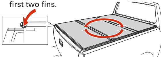
**3** Carefully refold the bed cover without shifting its position on the truck bed.
