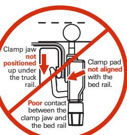
Ensure that each clamp is engaged on each side of the truck.
