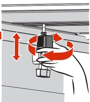
The optimal position of the clamp body is to match the bottom of the ridges to the bottom of the metal flange.
