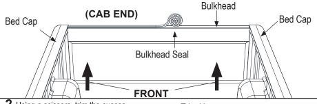
**2.**Using a scissors, trim the excess seal off where the seal meets the bed cap. Be sure <u>NOT</u> to cut the seal short of the bed cap, making sure the corner is sealed properly.
