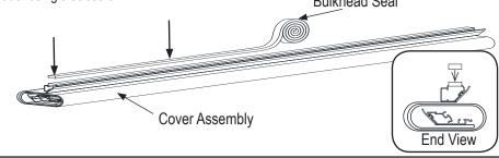
**2.** Turn the cover assembly right side up with the seals facing down. Place the cover assembly so the bulkhead seal sits on the bulkhead. Continue installation from the owner's manual.
