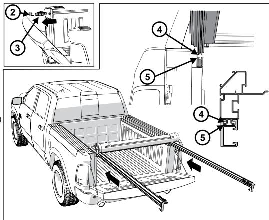
3.4 Slide the cover rail assembly forward so that the cab rail seals (6) make good contact with the installed
