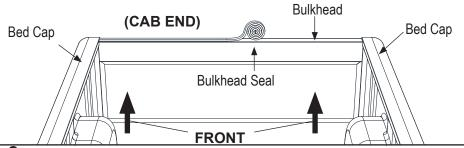
**2.** Using a scissors, trim the excess seal off where the seal meets the bed cap. Be sure <u>NOT</u> to cut the seal short of the bed cap, making sure the corner is sealed properly.
