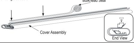
**2.** Turn the cover assembly right side up with the seals facing down. Place the cover assembly so the bulkhead seal sits on the bulkhead. Continue installation from the owner's manual.
