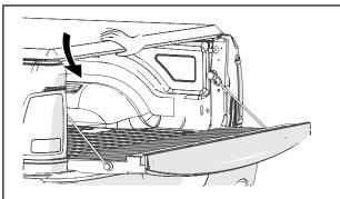
3. Roll up the cover. Do not disengage the hook and loop fasteners prior to rolling the cover.
