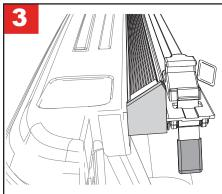
Position the driver side rail (A) against the truck bed rail. With the tailgate closed, slide the rail back until the rear seal is slightly compressed against the tailgate. Adjust the rail vertically so that the seal is flush with the truck bed caps.
