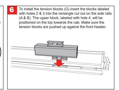
Secure the tension blocks to the side rails (A & B) by inserting the hitch pin (H) into hole number 2 on the underside of the side rails. If your covers tension is too tight or too loose simply remove the tension blocks and reposition. See chart on page 4 to fine tune your tension blocks once the cover is fully installed.
