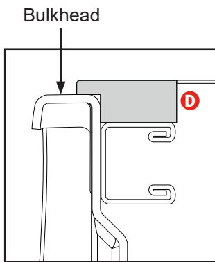
Side view of weather seal showing how the weather seal is positioned across the truck's bulkhead.
