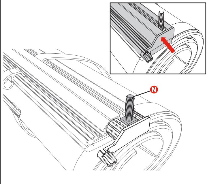
**13** Place the cover (C) on the side rails (A & B) towards the front of the truck bed (near the cab). The front header seal is designed to help shed water and should be sitting on top of the bulkhead.
