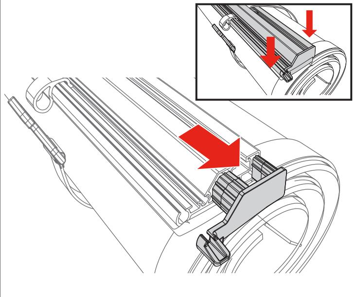
**12** **Install the bolts (N) by sliding them into the header as shown below.** Do this on both driver and passenger sides. Reinstall both end plugs as shown.
