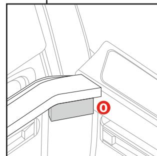
**4** Remove cargo rail end plugs: Begin by pushing in on the end plug tab and at the same time push the end plug out of the rail.
