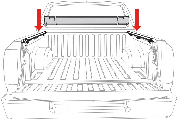
**14** To connect the cover to the rails (A & B) thread the plastic washers (L) and hex nuts (N) onto the bolts (M) attached to the cover (C). Tighten with a 9/16" wrench or socket. Do **NOT** overtighten. Repeat this process on the other side of the cover.
