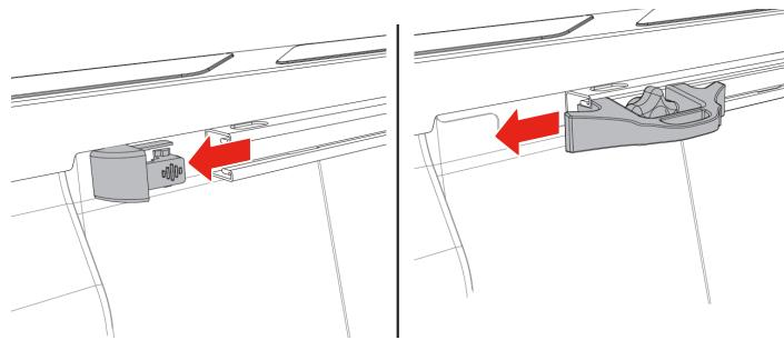
**5** Install 3 anchor blocks (E) into the accessory rail from the tailgate end. Then put the end cap back into the tailgate end of the accessory rail. Repeat installation for drive side.
