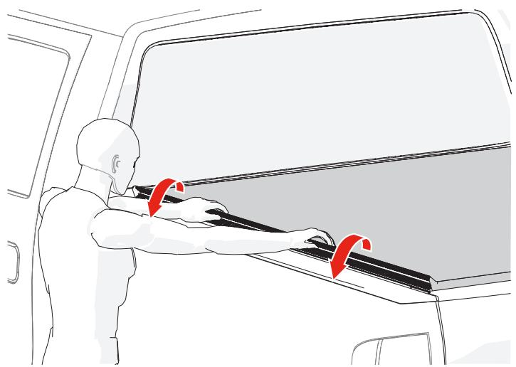
**18** Once the side of the hook and loop are engaged, use the palms of your hand to firmly push the loop strip into the hook track the entire length of the cover. This will prevent wind from lifting the cover and causing possible damage. Do this on both driver and passenger sides.
