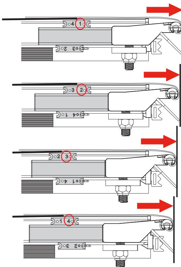
**Position 1** is set for maximum forward tension. The **NUMBER 1** is positioned on the top front. The hitch pin always goes into the bottom front hole.
