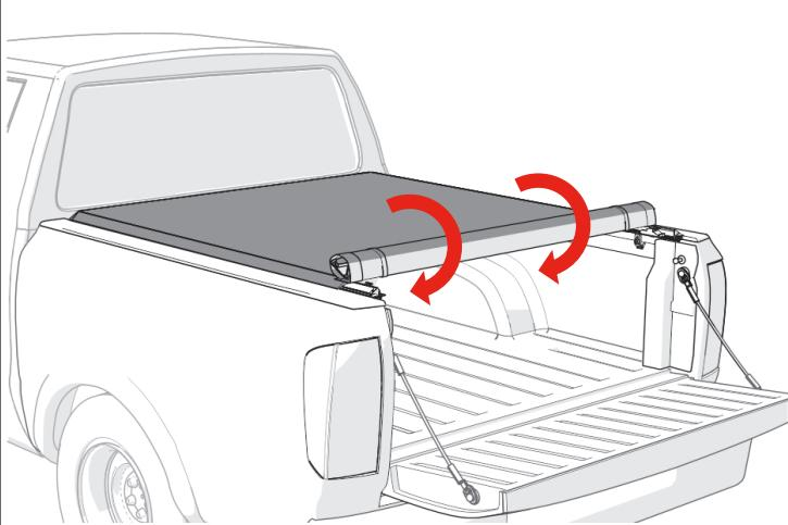
**16** Place the rear header into the header stops which are located on both side rails (A & B). Rotate the rear header downwards until you feel the cover latch in place. A clicking sound will indicate a correctly installed cover.
