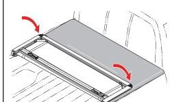
IMPORTANT: Before folding the second section of the tonneau, the rear clamps must be stowed into the rail to prevent damage to the fabric. Failure to stow the handle will puncture the tarp and void the warranty.
