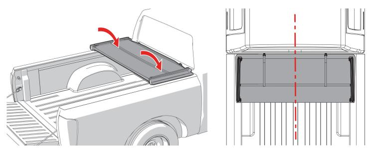
Unfold the bed cover fully and adjust the position over the truck bed for proper cab and tail alignment. Then carefully refold the bed cover without shifting its position on the truck bed. **NOTE**: Ensure the tail seal contacts the tailgate cap as shown.
