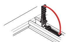
Fold the tonneau forward and fasten the straps in the middle section to the front rail. Check that the straps are tight. Failure to do so could allow the wind to blow the cover back resulting in damage to the
