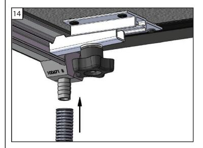
14. Attach the drain tubes to the fittings at the front of the bed rail and position the tubes to divert water out of the truck bed. This can be done by placing the tube behind a bed liner, through an existing hole in the bed, or by drilling a 5/8" hole in the bulkhead.
