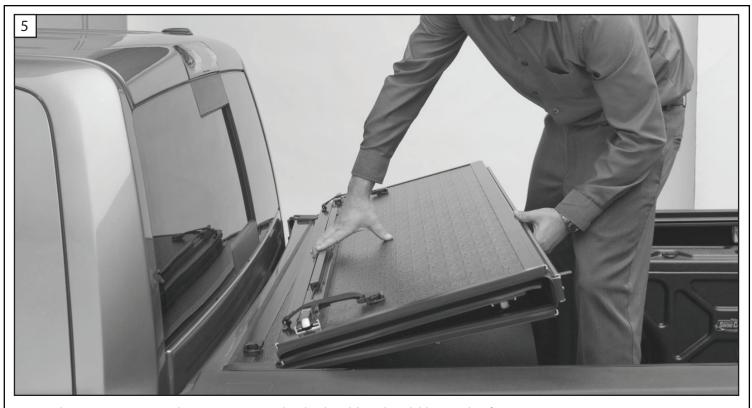
5. Set the tonneau onto the mounting rails, the buckles should be to the front.
