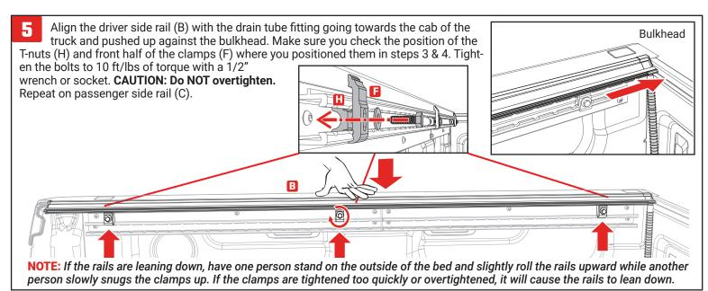
Without Utili-Track System: Attach three clamps (F) to the driver side rail (B) to the truck bed. Place the front clamp 6-8 inches from the bulkhead. Place the rear clamp as close to the tailgate as possible. Center the middle clamp accordingly. Clamps should be evenly spaced along the full length of the rail. Loosely tighten with a 1/2" wrench to make sure the clamps engage with the side rail. Repeat on the passenger side rail (C).
