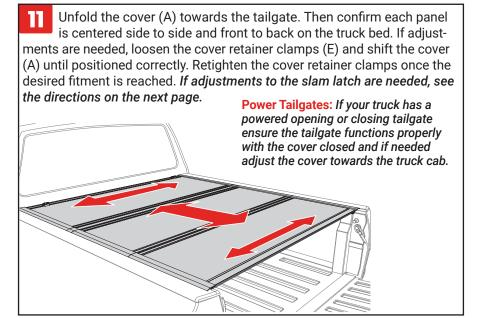
The rear edge of the cover (A) and tailgate seal should rest on top of the tailgate. You are ready to drive with your cover in the closed position.
