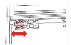
With the latch cover removed, loosen the screws and move the latch bracket to adjust. s the screws. Slide the latch housing back on.
