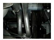
9) Place right side tailpipe **#16415S** into position over the axle and slip into the right side muffler outlet. Connect the hangers at the front and rear of the pipe to the rubber mounts on the vehicle. Install a provided 2 1/2" clamp onto the muffler outlet and tighten enough to hold, but still allow for adjustment.
