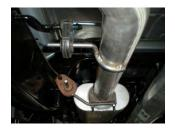
7) Connect the inlet of the muffler **#8530572-Z** to the inlet pipe. Use a stand to support the muffler and install clamp hanger **#392HA** provided in the parts kit onto the inlet of the muffler.
