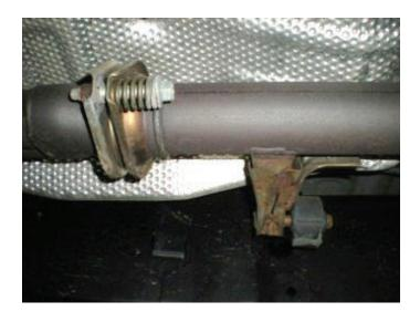
5. Separate hangers (x4) on muffler and front pipe assembly from rubber mounts on vehicle; then remove assembly from vehicle.
