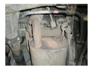
4. Remove factory spring loaded bolts (x2) at inlet pipe flange connection and set aside. Retain bolts and springs for later use.
