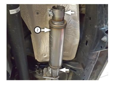
10. Route overaxle assembly (3) over axle and connect it to muffler then insert wire hangers in mounts. Place clamp (5) onto exit pipe assembly (4) and connect it to overaxle pipe. Tighten clamps enough for adjustment.
