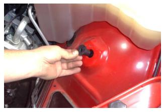
15. Insert 3/8-16 rubber well nut (3) in airbox mount hole in wheel well.
