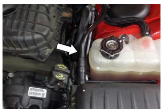
5. Carefully pull the hard plastic breather line from the hose on the airbox.
