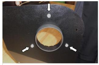
11. Assemble air filter adapter (31) to heat shield (28) using M6 screws (12), lock washers (11) and flat washers (10).
