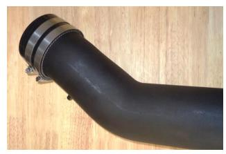
21. Install two small hose clamps (24) on straight coupler (23), and install coupler on throttle body end of tube. Do not fully tighten the hose clamps at this time.
