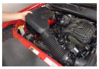
8. Carefully disconnect the intake duct from both the throttle body and the airbox, then remove it from the vehicle.
