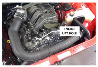
22. Install the intake tube in the vehicle. Leave hose clamps loose at this time. Note the engine lift hole behind bracket (16).
