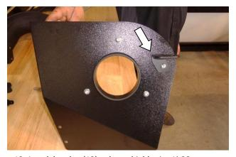
12. Attach bracket (13) to heat shield using ¼-20 screw (5) (against the bracket) and nut (7), lock washer (8) and flat washer (9) (against the heat shield). Do not fully tighten hardware at this time.
