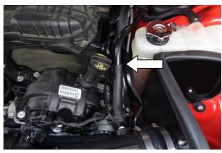
27. Cut the breather hose to the required length (i.e., to the lip on the hard plastic breather line), then push the hose onto the breather line (to the lip).
