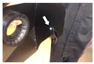
Attach bracket (4) to heat shield using ¼-20 screw
