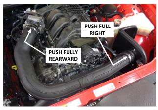
25. Push the straight coupler up against the throttle body. Push the flex coupler up against the heat shield. Then tighten all hose clamps.
