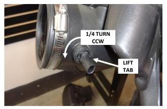
10. Remove the air temp sensor from the intake duct by lifting the locking tab, then turning the sensor a quarter-turn counter-clockwise. Then remove the o-ring from the sensor. CAUTION: The sensor is delicate! Handle it with care, and store it in a safe location until reinstallation.
