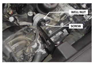
23. Insert 5/16-18 rubber well nut (19) in engine lift hole, then insert the 5/16-18 screw (17) through the bracket into the well nut. Tighten the screw until the well nut expands against the inside of the hole.
