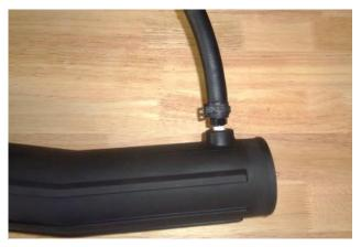
19. Install 5/8" ID hose (25) on the barbed fitting and secure with pinch clamp (26). (Install full length of hose; it will be cut to length later.)
