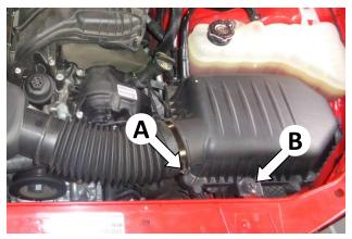
6. Loosen the hose clamp securing the air intake duct to the airbox (A). Remove airbox mount bolt (B) and retain for reinstallation at Step 16.
