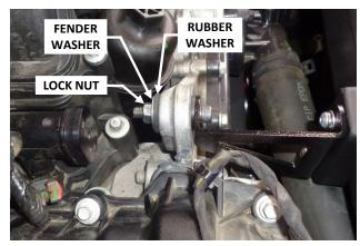
24. Install rubber washer (20), fender washer (21) and lock nut (22) hand tight on screw (17). Then tighten the 2 bracket screws (12). Finally, tighten locknut (22) while holding screw (17) stationary.
