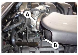
7. Loosen the hose clamp securing the air intake duct to the throttle body (A). Disconnect the air temperature sensor plug (B).
