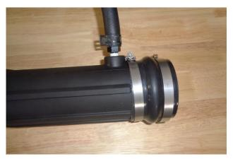
20. Install two large hose clamps (14) on flex coupler (29), and install coupler on airbox end of tube. Do not fully tighten the hose clamps at this time.
