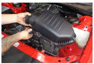
9. Remove the airbox from the vehicle.
