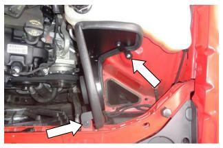
16. Place the assembled heat shield in the vehicle. Adjust the alignment of the brackets. Secure the rear bracket with 3/8-16 screw (6), secure the front bracket with stock bolt removed at Step 6, and tighten the bracket hardware.
