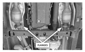
**4. Remove and retain 4 screws and springs** at the 2 catalytic converter flanges.
