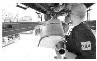
5. Disengage muffler rods from rubber isolaters (3 places), and remove muffler and pipe assembly from vehicle. Remove and retain 2 flange gaskets. Return the spare tire to its stowed position.
