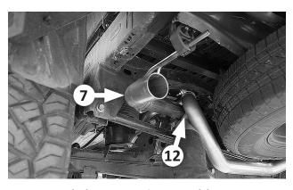
**14. Slip a clamp (12) over the left tailpipe (7).** Install its hanger rod in the rubber isolator, then slip it over the over-axle pipe. Verify 3" of insertion, and snug the clamp slightly.
