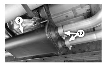
11. Slip two clamps (12) over the muffler's (3) inlets (the end with the hanger rods). Install the hanger rods in the rubber isolators, then install the muffler on the inlet pipes. Verify 2" of insertion, and snug the clamps slightly.
