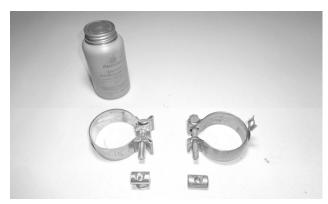
**6. Before installing clamps in the following steps,** remove their nuts, apply anti-seize compound to the bolt threads, and re-install the nuts.
