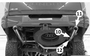
15. Slip a clamp (12) over the end of each side exit (9) or rear exit (10) pipe, and install each exit pipe on its tailpipe. Align each exit pipe as desired, verify 3" of insertion, and snug each clamp slightly. Install a tip (11) on each exit pipe. Align each tip as desired, and tighten its clamp.
