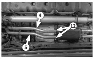
12. Slip a clamp (12) over the muffler's left outlet. Move the left over-axle pipe (5) into place, and insert its hanger rod into the rubber isolator. Insert the pipe into the muffler, verify 2" of insertion, and snug the clamp slightly. Repeat the process for the right over-axle pipe (4).
