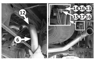
13. Slip a clamp (12) over the right over-axle pipe. Install the frame hanger (13) on the right tailpipe (6) hanger rod, with the flat pointing outboard and facing up toward the frame. Slip the tailpipe over the over-axle pipe. Then fasten the bracket to the frame with the bolt (14) and a flat washer (16) against the frame, and the other flat washer (16), lock washer (17), and the nut (15) against the bracket. Verify 3" of insertion, and snug the clamp slightly.
