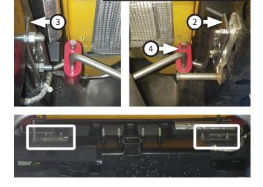
6. Connect **muffler (1)** to mid pipe, inserting wire hanger into rubber hanger. Adjust muffler to fit properly as shown then tighten clamp.
