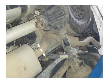
4. Support muffler then remove and retain flange fasteners. Disassemble wire hangers from isolators, disconnect inlet pipe and remove exhaust system.
