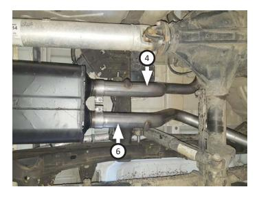
11. Place clamp (13) onto left rear tailpipe (5) then connect it to left overaxle pipe. Insert wire hanger into rubber hanger then tighten clamp just enough to allow for later adjustment.
