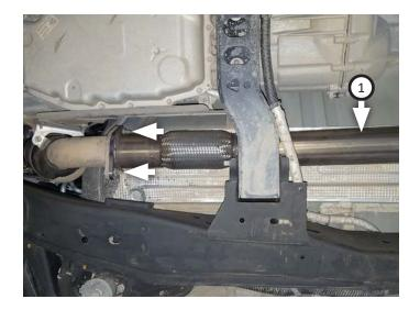
**NOTE:** If your vehicle has a 147" wheelbase, trim 10" from rear of extension pipe before completing this step.
