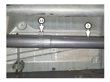
8. Place clamp (14) onto muffler (3) then connect it to extension pipe. Tighten clamp just enough to allow for adjustment then place (x2) clamps (13) onto muffler outlets.
