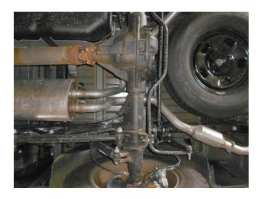
4. Disassemble wire hangers from isolators on muffler and inlet, then remove clamp on slip connection behind factory Y-pipe. Remove muffler and set aside.
