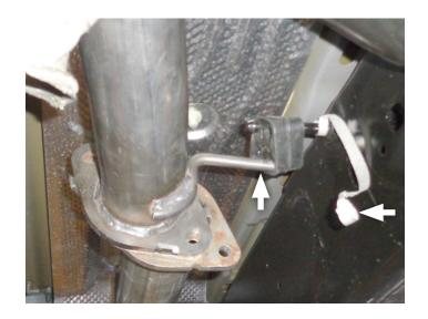
9. Secure flange with **bolt (3)**, (x2) **flat washers (4)**, **split lock washers (5)** and **nut (6)** through each hole.
