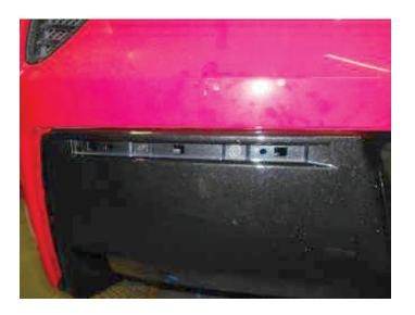
6. Remove hex bolts (x2) in cavity just above exhaust tips. With assistance, remove panel secured along top edge with clips. Grasp panel at one end through vertical slot, carefully pull it out and set it aside.
