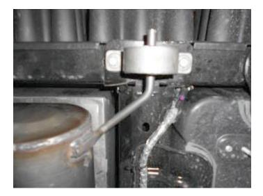
**NOTE:** Once actuator motors are removed from factory system, please note orientation of actuator lever. Do **NOT** turn or rotate levers.
