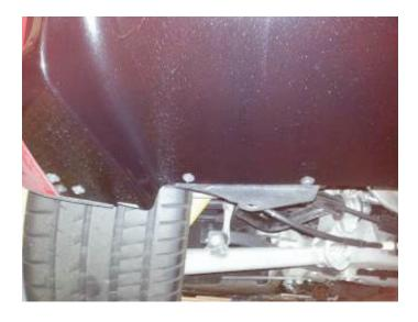
4. Carefully remove grates from bumper sides by releasing small clips. Below, where red and black panels touch, they clip together. Use a small flat blade screwdriver to carefully separate them.
