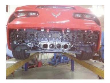
Find clamp connection on each pipe just forward of rear sub-frame and axles. Loosen nut on each clamp.
