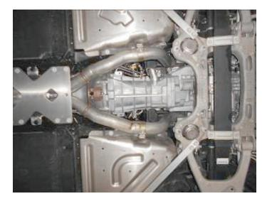
9. Disassemble both muffler assemblies by unbolting their hanger mounts, loosening front connection then pulling them out over axle. Transfer hanger mounts from factory to Outlaw mufflers and retain bolts for later.
