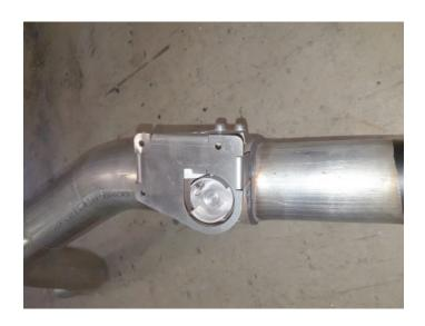
12. Route each muffler up and over axle into clamped connection then install final actuator onto front driver side valve. Secure assembly with fasteners and hanger mounts (removed step 9) to vehicle frame.
