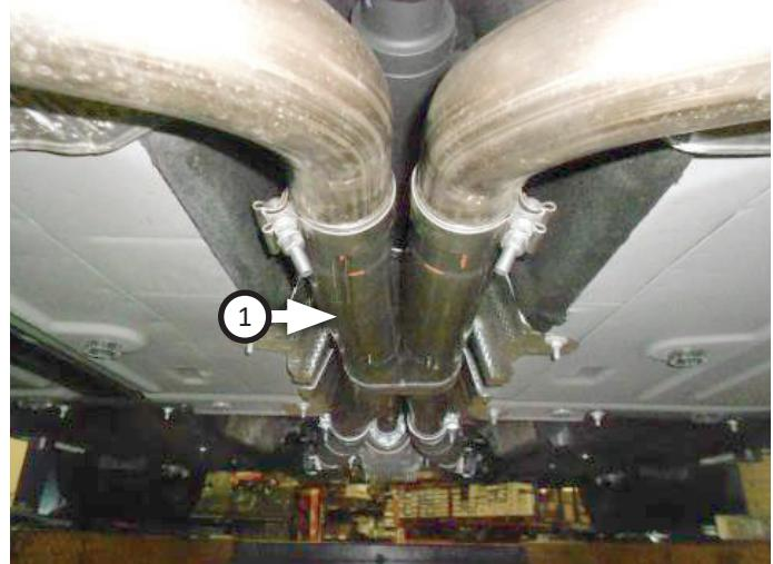
12. Place (x2) **clamps (6)** onto both **muffler (4)** inlets then connect them to scavenger pipe, sliding them  $1\frac{3}{4}$ " deep. Level mufflers and tighten clamps just enough to hold parts but still allow for adjustment.
