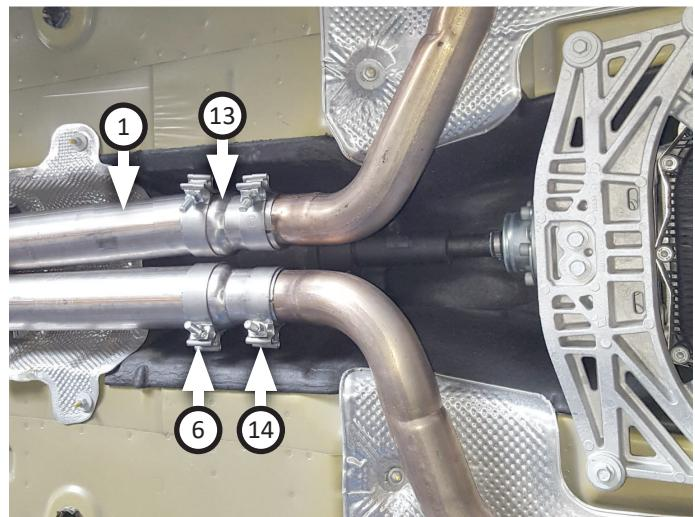
11. Place (x2) **clamps (5)** onto **scavenger pipe (1)** inlets then connect it to head pipes with offset outlet pipe oriented to passenger side). Level and center assembly in drive line tunnel then tighten clamps enough to hold parts.
