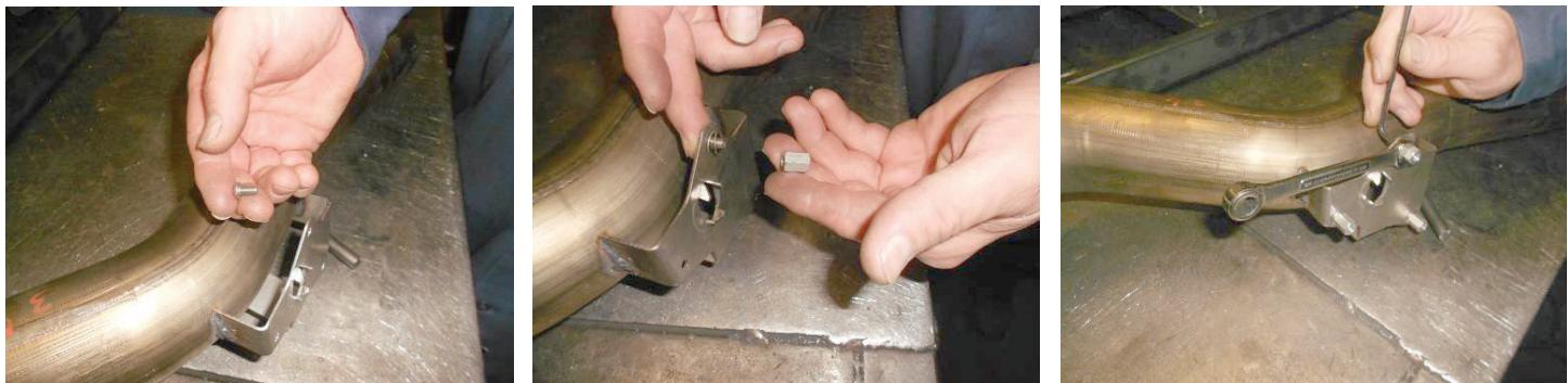
8. Complete step on both actuators and tailpipes: Place actuator on mount, with spring oriented between tabs then loosely attach it using (x3 ea.) **screw (10)** and **flat washer (12)**.
