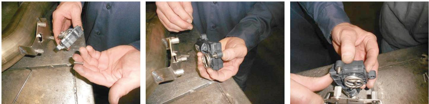
9. Complete step on both actuators and tailpipes: Ensure center arm of actuator spring sets between top and bottom mount tabs, then tighten (x3) screws securely.
