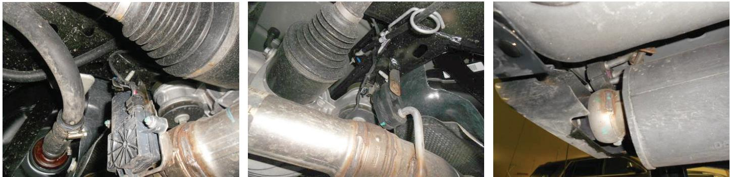
4. Remove (x3) nuts securing actuator to mounts then remove actuator and spring from mount on each tailpipe.
