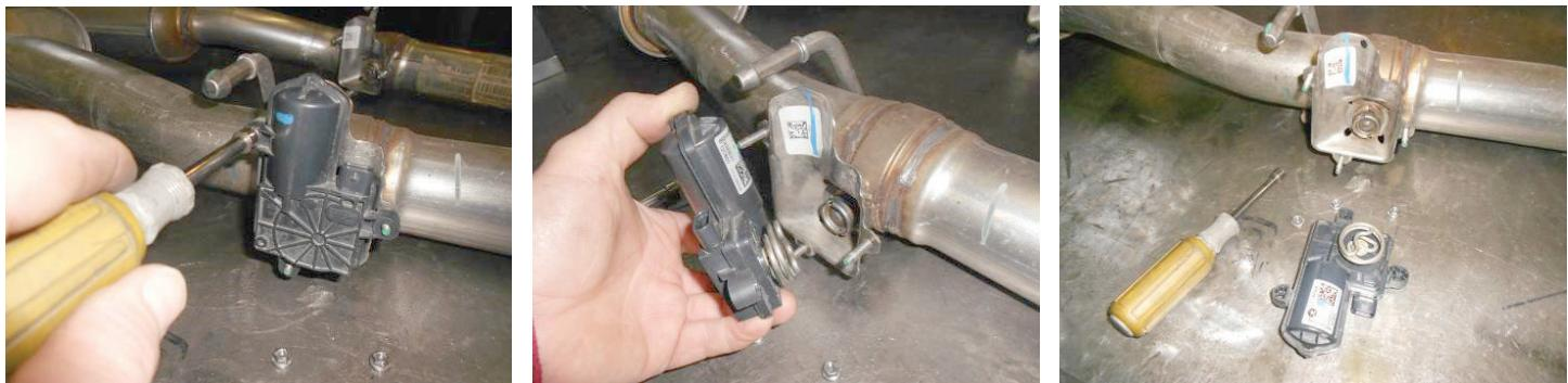
5. To install this kit properly, use standoffs sized to your vehicles' actuator valve springs (pictured below).
