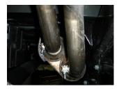
4) Place the provided 2<sup>1</sup>/<sub>4</sub>" clamps onto the muffler outlets and re-install the tailpipes into the muffler outlets. Be sure to line up the tabs on the tailpipes with the notches on the muffler outlets. Tighten the clamp securely.
