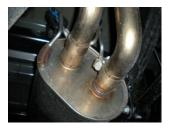
1) Loosen the two clamps at the back of the muffler and carefully slide the tailpipes toward the rear to remove from the muffler. Allow the pipes to hang until installation of the Flowmaster muffler.
