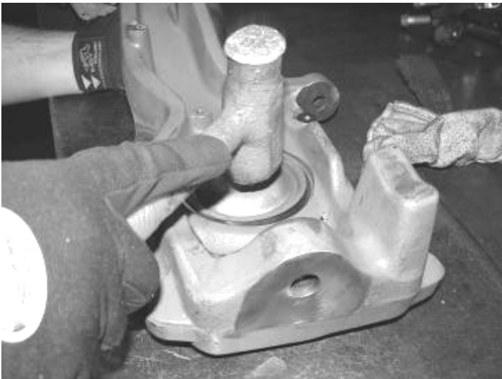
Photos above show removal and installation of the 2wd dust shield.
