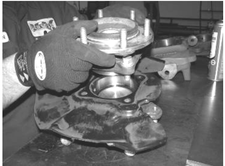
photo shows removal of hub with the backing plate already removed
