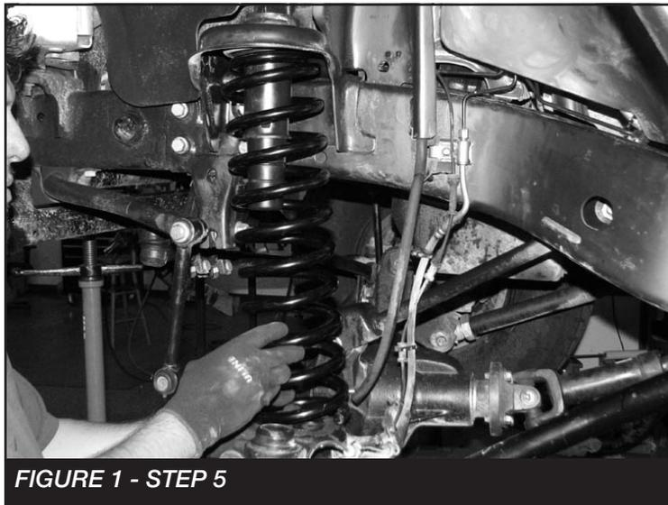
6. Refer to kit box instructions if installing new control arms. Reconnect the track bar and brake line brackets.
