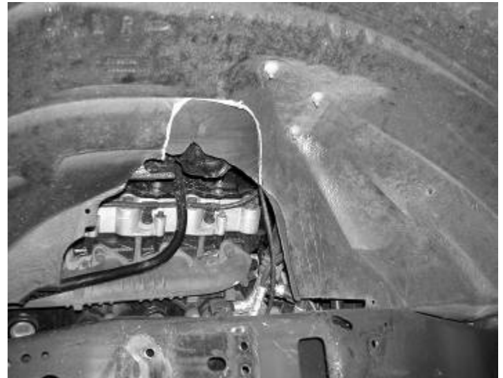
Passenger Side Marked and Uncut
