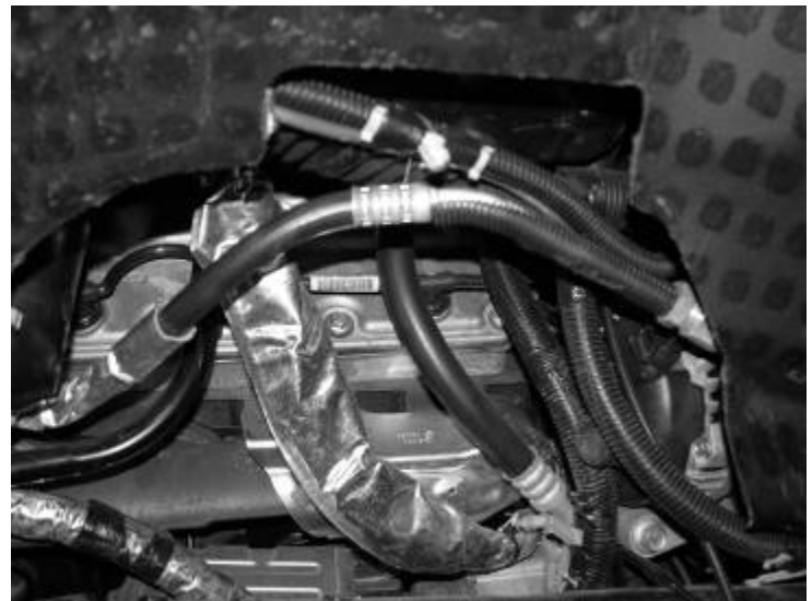
Photo shows bent A/C line
