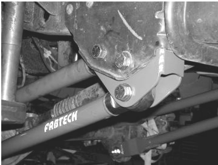
Assembly of the FT292 Alignment Cam
