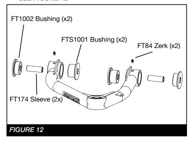
11. Install the upper arm using the factory hardware. Place the new FT58-1 washers on the inside and outside of the bushings. When installing the arm on the truck make sure the barrel gussets are up. Torque to 120 FT-LBS. SEE FIGURES 13-14
