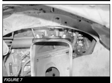
7. Install the FT825252 or FT820252 Coilover into the new upper mount using the ½-13 x 2-¼ bolt from the shock hardware. Torque 90 FT-LBS. **SEE FIGURES 8-10**
