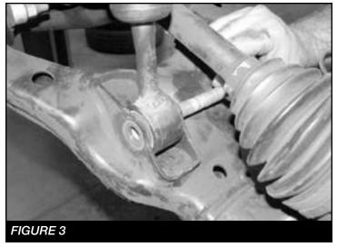
5. Using 1-1/2" Barrel sander, sand a small notch in the lip at the top of the bucket. The radius should be on both sides of the bucket parallel to the front of the bucket. This radius is to add clearance the shock pivot bolt.
