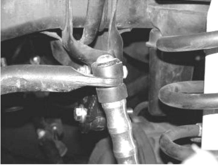
20. Attach the brake line tab back to the original mount using the original hardware. You may need to pull the factory hose through the bracket to gain some slack. Repeat this on the opposite side of the truck.
