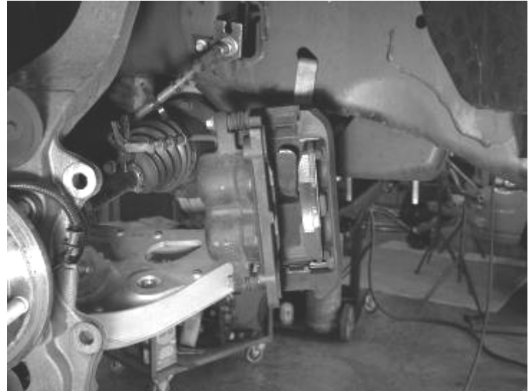
Brake Caliper Shown Hung from Frame
