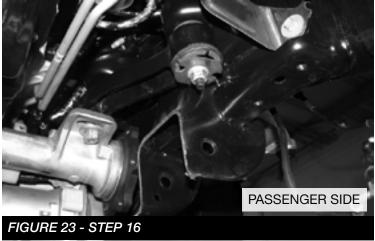
16. Locate the factory front lower control arm pockets. Grind about 1/4" from both corners on both pockets. NOTE: The bracket located on the passenger side that holds factory skid plate on will need to be cut off. SEE FIGURES 24-25
