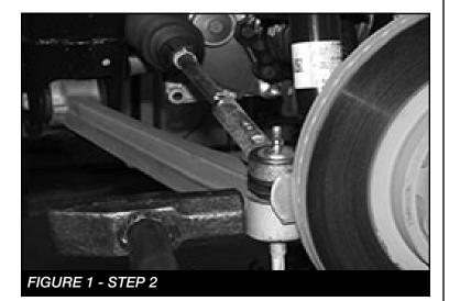
Remove the brake hose bracket from the steering knuckle and coil bucket, save hardware. Remove the caliper from the rotor and secure the brake caliper to the frame out of the way. DO NOT ALLOW THE BRAKE CALIPER TO HANG FROM THE HOSE. SEE FIGURES 2-3
