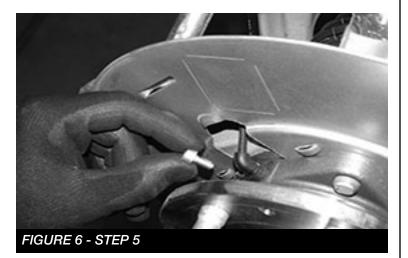
6. Remove the axle nut and washer, save for re-installation. **SEE FIGURE 7**
