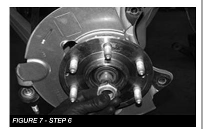
7. Loosen the upper and lower ball joint nuts. Using a large hammer, carefully strike the spindle at the ball joint to dislodge the ball joint. Use care not to hit the ball joints when removing. **SEE FIGURES 8-10.** Remove and save the nuts. Discard the factory spindle.
