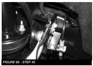
46. Re-route the brake hose and the ABS line to the steering knuckle. Secure the ABS line to the back of the knuckle using the provided clamp and 1/4" bolt and washer. Torque to 10 ft-lbs. Re-connect the ABS line into the hub assembly and torque to 10 ft-lbs. Use the provided black zip ties to mount the brake line in a safe location. **SEE FIGURES 69-70**
