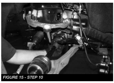
Loosen and remove the lower control arm bolts. Remove control arms and set aside with hardware. SEE FIGURES 16-17
