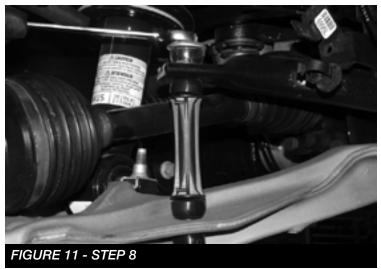
Remove and save the upper coilover assembly nuts, and lower bar pin bolts. Remove the coilover. NOTE: For Magneride models disconnect the wire at the top of the coilover. SEE FIGURES 12-14.
