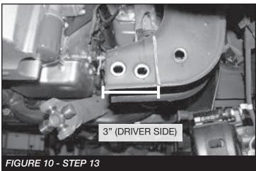
14. Locate the rear passenger lower control arm mount on the frame. Measure 3 ½" from the inside edge of the mount toward the frame and mark with a paint pen. Use a sawzall and cut the mount from the frame.
