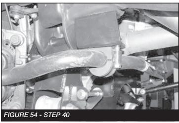
41. Locate FT20602 Sway Bar Mounts and the supplied 18mm x 50mm hardware. Position the Sway Bar Mount so that it is on the bottom of the sway bar with the SHORTER side of the mount against the stop plate end of the mount. Attach with the 18mm hardware and torque to 300 ft-lbs. Locate the factory sway bar end links and attach to the new mount and the lower control arm. (NOTE - SOME PICK UP TRUCKS MAY BE EQUIPPED WITH SUV STYLE SWAY BAR). SEE FIGURE 55
