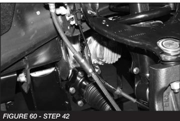
43. Re-route the brake hose and the ABS Line to the steering knuckle using the adel clamp to the back of the steering knuckle and attach with ¼" x 3/4" bolt and washer. Torque to 10 ft-lbs. Route the ABS line next to the brake hose. Re-connect the ABS line to the harness in the wheel well. Using provided plastic zip ties, secure line to the hose and away from the tire and wheel. **SEE FIGURE 61**
