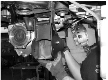
26. Attach the rear Diff mount (FT20486) to the last open mounting tab on the Factory Diff using a ½"-13 x 3" bolt, washers, and lock nut. Toque all the hardware to 127 ft-lbs. SEE PHOTO BELOW
