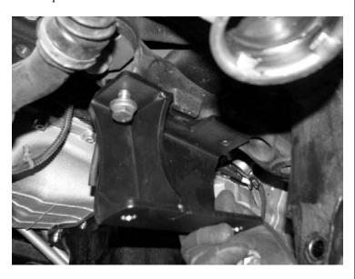
19. Locate and install the Fabtech Pass side Diff bracket (FT20477) to the bottom of the factory frame mount using the factory hardware. SEE PHOTO BELOW
