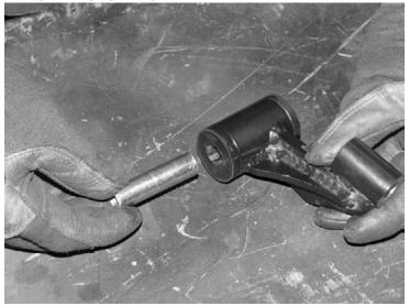
24. Install the Rear Diff bracket (FT20486) into the mount on the rear crossmember (FT20475BK). Use the ½"-13x4" bolt and the FT30201 nut tab to secure the bracket to the cross member. Leave loose. SEE PHOTO BELOW
