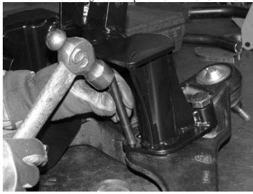
33. Remove the torsion bar bracket and drill a 1/2" hole. SEE PHOTO BELOW
