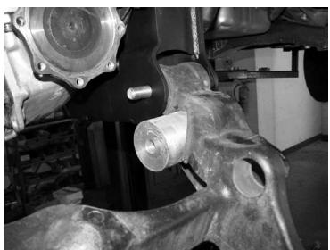
30. Locate the medium aluminum RTS bushing (FT20482) an install it into the back side of the torsion bar socket in the lower control arm. SEE PHOTO BELOW
