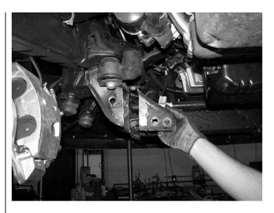
16. Locate the pass. lower control arm pocket and cut out the 3" section over the holes on the front side of the pocket. SEE PHOTO BELOW
