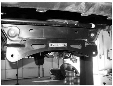
28. Locate the factory lower control arms and remove the lower shock mount bushing using a ball joint press tool. SEE PHOTO BELOW
