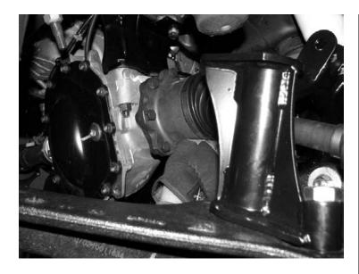
44. Locate the o-ring, dust shield and hub. Install into the Fabtech spindle. Torque the factory hub bolts 184 ft-lbs. Install the axle nut and torque to 165 ft-lbs. Replace axle nut cover. SEE PHOTOS BELOW
