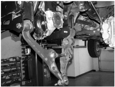
35. Locate the Torsion Bar mount for the Driver side lower control arm (FT20806). Install the torsion bar relocator to the arm using the supplied hard ware ½"–13 x 7-1/2", ½"-13 x 1-3/4", 5/8"-11 x 7-1/2", M18-2.5x70mm., washers and lock nuts. Reference the diagram above step 29 for all the torque specifications for the torsion bar bracket. SEE PHOTO BELOW
