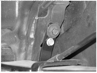
56. Locate and install the rear lift blocks with the provided short center pin on the bottom of the block, to the axle. The integrated bump stop should face to the inside of the vehicle. Using the provided U bolts, nuts and washers align axle, lift blocks, and springs and torque to U Bolts to 317 ft-lbs. SEE PHOTO BELOW.
