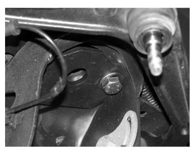
38. Install the front shock (FTS7338) or (FTS6338) with the stem in the upper  $\,$  mount. SEE PHOTOS BELOW
