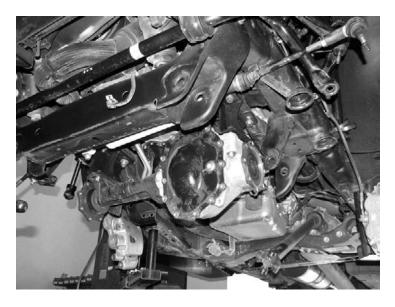
21. Check this area of the frame after installing the Diff. You may need to add a small amount of clearance for the CV. SEE PHOTO BELOW
