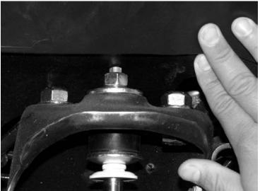
39. Install the lower mount of the shock into the rear shock mount on the torsion bar bracket that is mounted to the lower control arm. Use a ½"-13 x 2-3/4" bolt, washers and lock nut. Torque to 127 ft-lbs. SEE PHOTO BELOW
