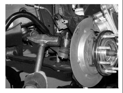
7. Remove the brake hose bracket from the top of the steering knuckle. Remove the caliper from the rotor and place above the upper control arm during this portion of the installation. Remove brake rotor from the steering knuckle. Unbolt the wheel speed sensor connection from the hub and control arm. SEE PHOTO BELOW
