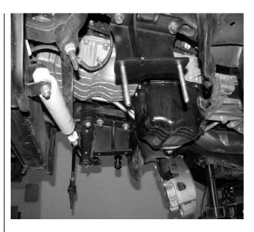
20. Locate the stock differential and reinstall with the 2ea ½"-13 x 3-1/2" bolts, washers and lock nuts on the driver side and the 2-½"-13 x 1-1/2" bolts, washers and lock nuts on the pass side. Torque all the bolts to 127 ft-lbs. SEE PHOTOS BELOW
