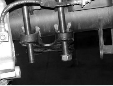
57. Install Fabtech shock part number FTS7333 or FTS6240 (not included) with the factory hardware and one 9/16" washer per side on both upper and lower mounts. Torque to 65 ft-lbs. SEE PHOTO ON NEXT PAGE.
