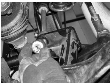
47. Remove the factory brake line bracket by either carefully cutting it off or bending it apart. Next, Install the front brake line extension bracket (FT20520) with the factory hardware and supplied 5/16" hardware. Clamp the ABS and brake line to the spindle using the supplied adel clamps and ¼" bolts. SEE PHOTOS BELOW
