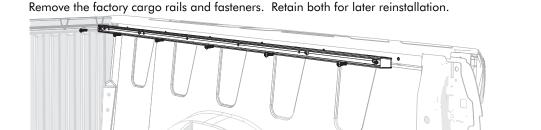
Align and slide the cover rail brackets into the slot in the rail. The brackets will be spaced to match the factory cargo rail holes.
