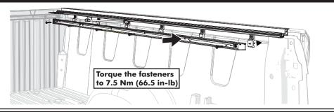
Repeat all of the steps for both sides. Return to the standard installation instructions. Follow step 2 for the bulkhead seal, then skip to step 8.
