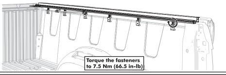
Mount the factory cargo rail to the lower holes of the cover brackets using the provided small fasteners.
