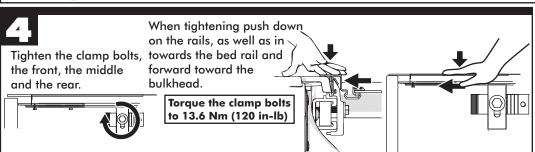
Repeat all of the steps for both sides. Return to the standard installation instructions. Follow step 2 for the bulkhead seal, then skip to step 8. Torque the clamp bolts to 13.6 Nm (120 in-lb)
