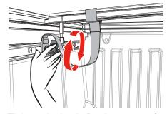
Tighten the knob. Do these steps for both the driver and passenger sides.
