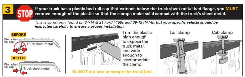
Ensure that the clamp is positioned under the metal bed flange. Hand tighten until clamp contacts the flange, then tighten an additional two turns.
