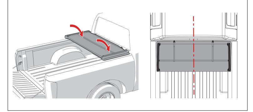
**5** Unfold the bed cover fully and adjust the position over the truck bed for proper cab and tail alignment. Then carefully refold the bed cover without shifting its position on the truck bed. **NOTE**: Ensure the tail seal contacts the tailgate cap as shown.
