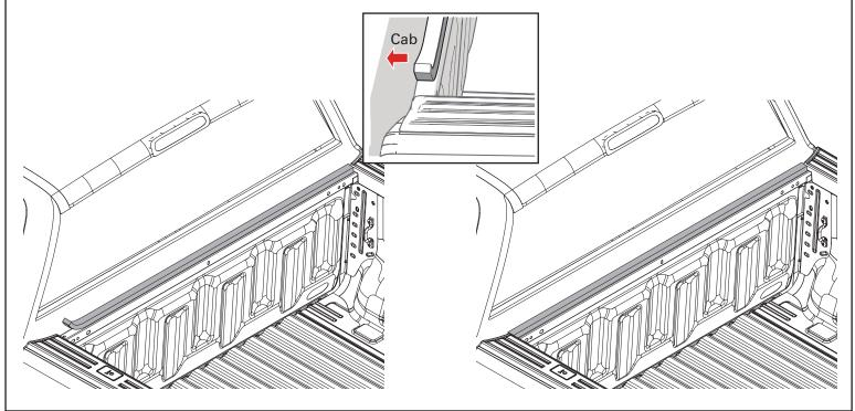
Place the assembled bed cover (A) over the cab end of the truck bed. **NOTE**: Take care not to damage or deform the seals when installing the bed cover onto the truck bed. Visually check to ensure the front bed cover frame is even on both sides and square with the bed. Make sure the cover is centered on the bed of the vehicle before tightening clamps.
