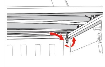
Hand tighten the clamps to hold the cover in position.
