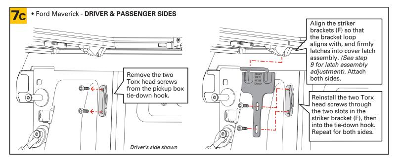
Adjustments and tightening of the latch assembly is required.
