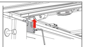
Align the striker brackets (C) so that the bracket loop aligns with and firmly latches into the cover latch assembly *(see step 8 for latch assembly adjustment).* Attach to both driver and passenger sides. Using the provided T-27 Torx wrench, tighten the screws firmly while continuing to align the latches in later steps.
