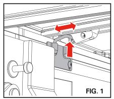
The bed cover latch assemblies and rotary knob come from the factory only partially tightened to allow for installation adjustments. Both latches and rotary knob will require adjustment and final tightening. **Only use the hand tools provided, do not use power tools**.
