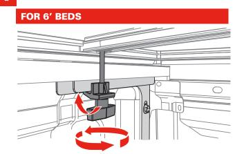
Hook the cab clamp under the installed cab rail brackets (G). Tighten the knob until the jaw makes contact, then turn an additional two turns. Repeat on the opposite side of the truck bed.
