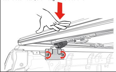
The tethers come installed looped over the bed cover bow with a clamp at the other end. Install the clamp end by sliding the clamp onto the truck rail. Make sure the clamp is positioned as far up onto the rail as possible. Firmly hand tighten the knobs. Install the tethers on both sides of the cover.
