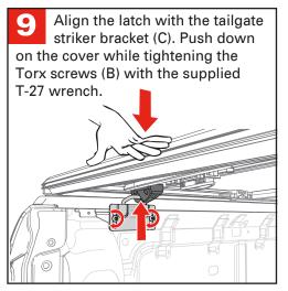
Adjustments and tightening of the latch assembly is required.
