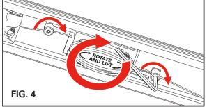
Double-check that the cover is secure and tight to the truck bed by gently lifting the corners to ensure the mechanisms are engaged.
