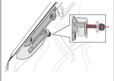
Attach the striker bracket (C) to the latch bracket (D) using the Torx head screws (B). Leave them loose for later adjustments.
