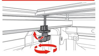
Hook the cab clamp under the truck bed rail metal flange. Tighten the knob until the jaw makes contact, then turn an additional two turns. Repeat on the opposite side of the truck bed.
