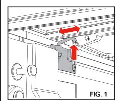
The bed cover latch assemblies and rotary knob come from the factory only partially tightened to allow for installation adjustments. Both latches and rotary knob will require adjustment and final tightening. **Only use the hand tools provided, do not use power tools**.
