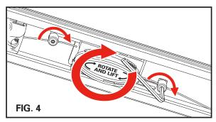
Double-check that the cover is secure and tight to the truck bed by gently lifting the corners to ensure the mechanisms are engaged.
