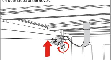
Close the tailgate and unfold the cover. Check that the cover is parallel and square with the truck bed and bed rails. If not parallel or square, open the cover and loosen the cab clamps to reposition the cover. Adjust and re-tighten both clamps.
