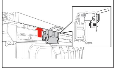
with the bed cover latch. Push down on the cover while tightening the Torx screws (E).
