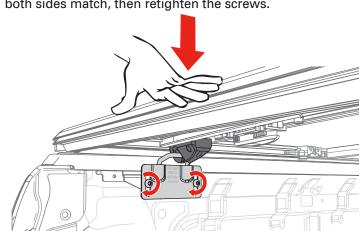
The tethers come installed looped over the bed cover bow with a clamp at the other end. Install the clamp end by sliding the clamp onto the truck rail. Make sure the clamp is positioned as far up onto the rail as possible. Firmly hand tighten the knobs. Install the tethers on both sides of the cover.
