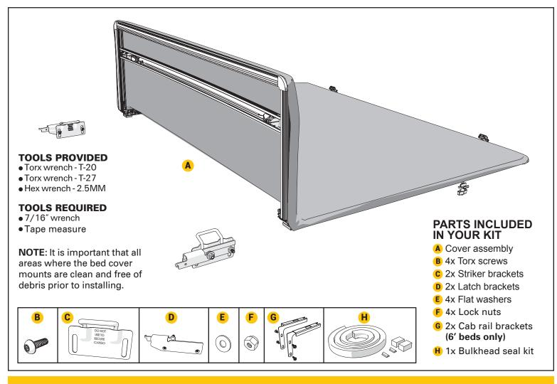
**IMPORTANT:** Please install the bulkhead seals (H) (for 5' & 6' beds) and the 2 cab rail brackets (G) (for 6' beds only) before proceeding. Separate installation sheets are found in the hardware bags.
