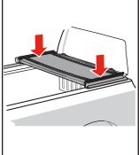
Unfold the bed cover (A) fully and adjust position over the truck bed for proper front (cab) and rear (tailgate) alignment. When positioned front and back, the tailgate seal should contact the tailgate with the first two fins.
