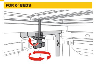
Hook the cab clamp under the installed cab rail brackets (G). Tighten the knob until the jaw makes contact, then turn an additional two turns. Repeat on the opposite side of the truck bed.
