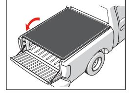
Align the latch with the tailgate striker bracket (C). Push down on the cover while tightening the Torx screws (B) with the supplied T-27 wrench.
