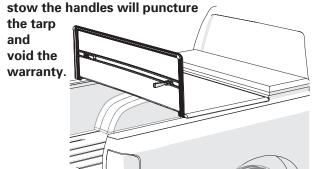
Fold the cover forward and fasten the straps to the front rail. Check that the straps are tight.
