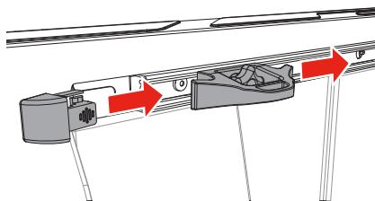
Reinstall any tie-down cleats and the end cap on both sides of the truck.
