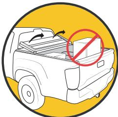
**Never operate the vehicle with a partially folded up cover.**
