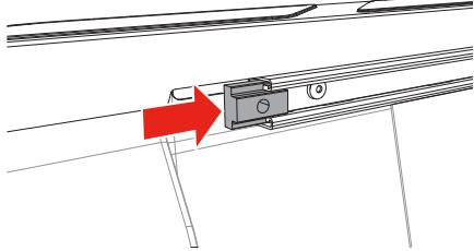
Insert the provided slide block into the cargo rail.
