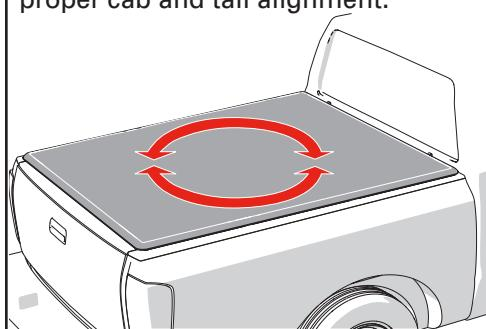
Then carefully refold the cover without shifting its position on the truck bed.
