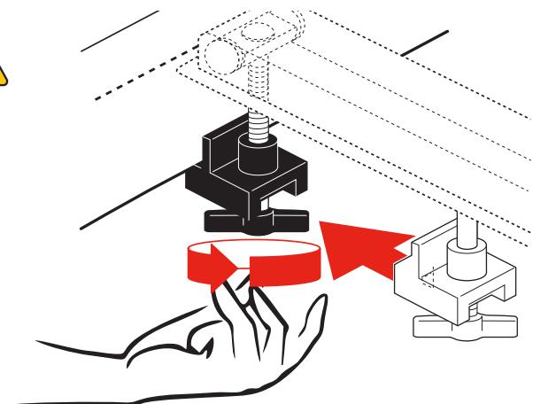
**5** With the tailgate open and the front (cab) clamps secure, completely close the cover
