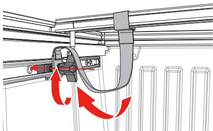
Thread the tether knob through the lock washer, through the tether bracket and into the slide block.
