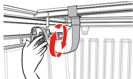
**!** Tighten the knob securely so that the tether clamp does not slide/shift or lift from the truck bed flange. Do these steps for both the driver and passenger sides.
