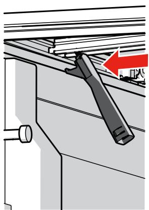
The clamps should be slid, at a slight angle, as far over to the rail as possible.
