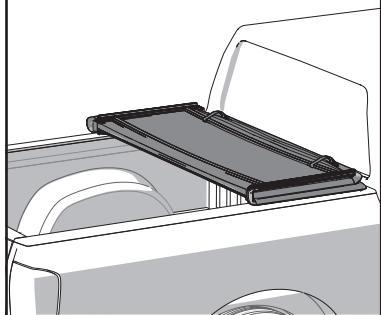
**2** Unfold the cover fully and adjust the position over the truck bed for proper cab and tail alignment.
