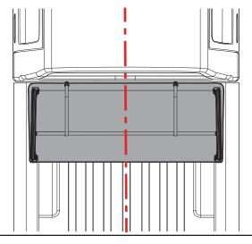
Ensure that the clamp is positioned under the previouly installed bracket. Hand tighten until clamp contacts the bracket, then tighten an additional two turns. **DO NOT** secure to only the lip of the bedliner or the plastic bed cap.
