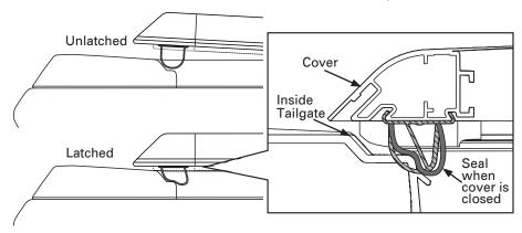
The rear (tail) clamps are stowed in the cover rail. Rotate the clamp down and slide it to the truck bed rail. The clamps should be slid, at a slight angle, as far over to the rail as possible. Pull the clamps straight down and release them to hook under the bottom of the metal bracket. Always latch the clamps on both sides of the bed.
