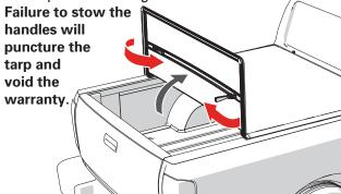
Fold the cover forward and fasten the straps to the front rail. Check that the straps are tight
