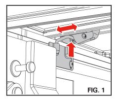
The bed cover latch assemblies and rotary knob come from the factory only partially tightened to allow installation adjustments. Both latches and rotary knob will require adjustment and final tightening. **Only use the hand tools provided, do not use power tools**.
