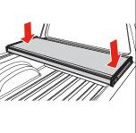
Unfold the bed cover (A) fully and adjust position over the truck bed for proper front (cab) and rear (tailgate) alignment. When positioned front and back, the tailgate seal should contact the tailgate with the first two fins.
