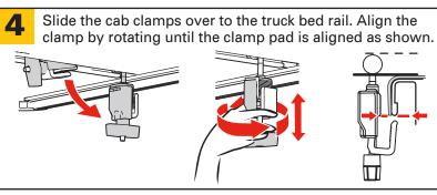
Push the clamp to the truck bed rail, rotate the jaw up under the rail and tighten.
