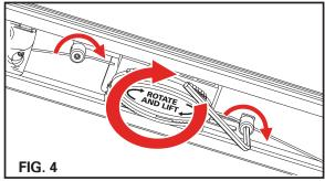
To make the final adjustment, loosen the striker bracket bolts or screws. Then move the bracket (C, F, H, or Q) down by firmly pushing the cover (A) to the truck rail and tailgate. Make sure that both sides match, then retighten all the screws while maintaining the pressure on the cover.
