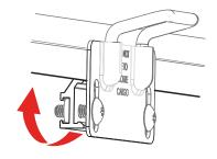
With the truck bed cover (A) closed, attach the striker brackets (C) to the metal truck bed rail.
