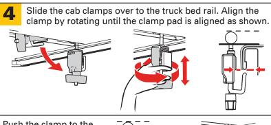
Push the clamp to the truck bed rail, rotate the jaw up under the rail and tighten.
