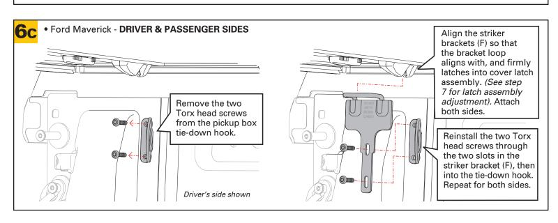
Adjustments and tightening of the latch assemblies are required.
