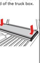
Unfold the bed cover (A) fully and adjust position over the truck bed for proper front (cab) and rear (tailgate) alignment. When positioned front and back, the tailgate seal should contact the tailgate with the first two fins.
