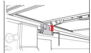
Align the striker brackets (C) so that the bracket loop aligns with and firmly latches into the cover latch assembly (see step 8 for latch assembly adjustment). Attach to both driver and passenger sides. Using the provided T-27 Torx wrench, tighten the screws firmly while continuing to align the latches in later steps.
