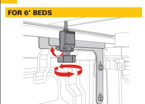
Hook the cab clamp under the installed cab rail brackets (G). Tighten the knob until the jaw makes contact, then turn an additional two turns. Repeat on the opposite side of the truck bed.
