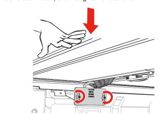
The tethers come installed on the bed cover hinge with a clamp at the other end. Install the clamp end by sliding the clamp onto the truck rail. Make sure the clamp is positioned as far up onto the rail as possible. Firmly hand tighten the knobs. Install the tethers on both sides of the cover.
