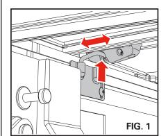
The bed cover latch assembly and rotary knob comes from the factory only partially tightened to allow for installation adjustments. **Only use the hand tools provided, do not use power tools**.
