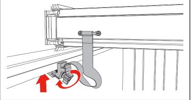
**20** Install the striker bracket (B) by loosening the Torx screws (E) until there is enough space for the backing plate (C) to fit behind the adapter rail (H) while the striker bracket plate (B) fits on the front of the adapter rail (H).
