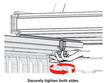
19 Close the tailgate and unfold the cover. Check that the cover is parallel and square with the truck bed and bed rails. If not parallel or square, open the cover and loosen the cab clamps to reposition the cover. Adjust and re-tighten both clamps.
