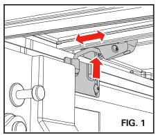
The bed cover latch assembly comes from the factory only partially tightened to allow for installation adjustments. **Only use the hand tools provided, do not use power tools**.
