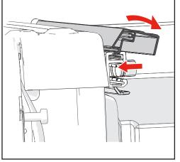
Before the adapter rail (H) is slid completely to the bulkhead, remove the backing and attach a rail end seal (J). Do this for both sides.
