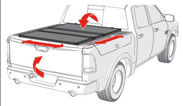
**21** Close the cover (A) and align the striker bracket (B) with the bed cover latch. Push down on the cover while tightening the Torx screws (E).
