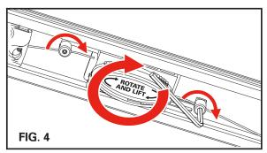
To make the final adjustment, loosen the striker bracket screws. Then move the bracket down by firmly pulling the cover to the truck rail and tailgate. Make sure that both sides match, then retighten the screws to 8 ft-lbs (10.8 Nm). Do this for both sides of the truck.
