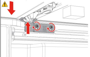
The tethers come installed on the bed cover hinge with a clamp at the other end. Hook the tether onto the truck bed tie-down. Install the tethers on both sides of the cover.
