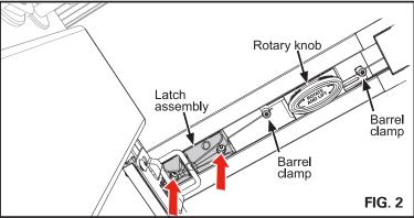
Rotate the rotary knob until you see the flat head screws. Tighten the two screws using the provided Torx T-20 wrench, (Fig. 3) so the knob does not move in the channel. Repeat on the other side.
