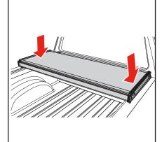
Unfold the bed cover (A) fully and adjust position over the truck bed for proper front (cab) and rear (tailgate) alignment. When positioned front and back, the tailgate seal should contact the tailgate with the first two fins.
