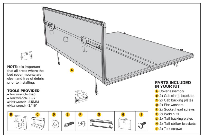
Place the folded, cover on the cab end of the truck bed. Make sure the cover is square with the truck bed and the bulkhead seal sits on the truck bed bulkhead.
