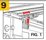
Adjustments and tightening of the latch assembly is required. The bed cover latch assembly comes from the factory only partially tightened to allow for installation adjustments. Only use the hand tools provided, do not use power tools.
