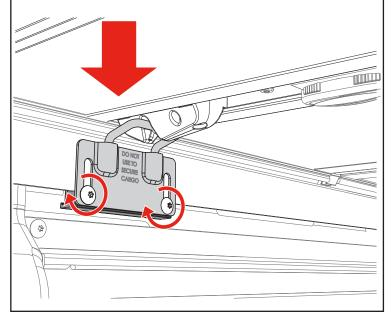
Opening the cover Open the cover by twisting the actuator knob and lifting the cover.
