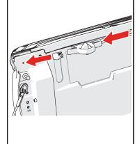
Install the cab slide block (B) into the rear (tailgate) end of the cargo rail. Position near the cab. Align the cab clamp bracket (C) with the cab clamp of the bed cover. Use the Torx screws (D) to mount the cab clamp bracket (C) to the cab slide block (B). Tighten the screws with the T-27 Torx tool. Do this for both sides of the truck bed.
