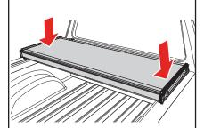
Unfold the bed cover (A) fully and adjust its position over the truck bed for the proper front (cab) and rear (tailgate) alignment. When positioned front and back, the tailgate seal should contact the tailgate with the first two fins.
