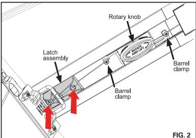
Rotate the rotary knob until you see the flat head screws. Tighten the two screws using the provided Torx T-20 wrench, (Fig. 3).
