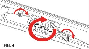
To make the final adjustment, loosen the striker bracket nuts (E). Then move the bracket (F, G) down by firmly pulling the cover (A) to the truck rail and tailgate. Make sure that both sides match, then retighten the nuts.
