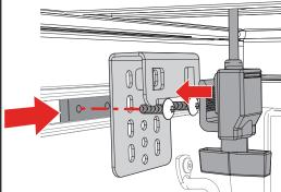
Hook the cab clamp under the cab clamp bracket (C) and tighten the T-handle until it contacts the bracket (C), then tighten two more turns. Do this for both sides of the truck bed.
