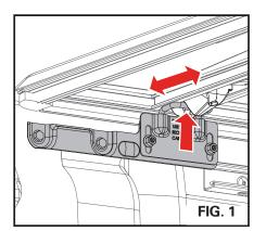
The bed cover latch assembly and rotary knob comes from the factory only partially tightened to allow for installation adjustments. **Only use the hand tools provided, do not use power tools**.
