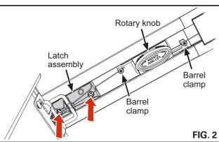
Rotate the rotary knob until you see the flat head screws. Tighten the two screws using the provided Torx T-20 wrench. (Fig. 3)
