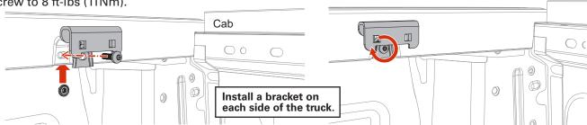
Remove the factory flange bolt, place the rear latch bracket (C) as shown and replace the factory flange bolt along with installing a Torx screw (F). Tighten the factory bolt (T-45) to 16 ft-lbs (22Nm) and the Torx screw (T-30) to 8 ft-lbs (11Nm).
