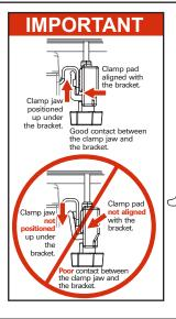
The optimal position of the clamp body is to match the bottom of the ridges to the bottom of the bracket.
